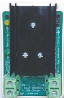
SC-2030 Solar Charger Usually located near batteries connected to TM-2030 with telephone cable.
