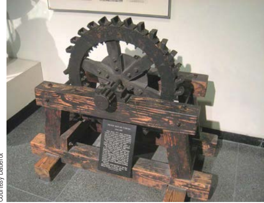
A Pelton impulse turbine, circa 1880, built by the Miners Foundry of Nevada City, California.
